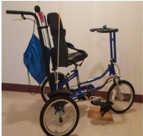
**FRE DCP16:** This tricycle is small enough for an average 7-year-old, but adaptable to fit most kids in their early teens. Direct drive and low gear ratios make pedaling easy for a beginner, yet challenging for and aggressive rider. Inseam 20"-26" maximum of 150lbs
