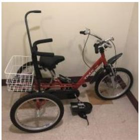
**TRIAD TMX T-5:** Is a robust tricycle for older children, it is fitted with 20" wheels and has a caliper brake with parking brake feature. It is suitable for children with an overall height of 47" (120cm) to 57" (145cm) and maximum recommended weight is 150lbs.
